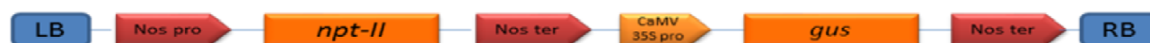
Fig.1b. Structure of expression vector: T-DNA region of pBI 121, containing I) transcriptional fusion of NOS promoter with the coding region of npt-II and NOS terminator II) transcriptional fusion of CaMV 35S promoter with the coding region of gus and NOS terminator
