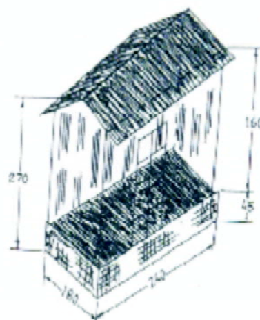
Fig.6 Onion Storage Structure Made of Thatch (Type-6)
